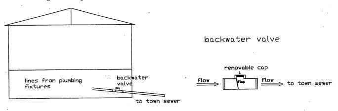
The Backwater Valve should be installed in the basement down stream of any other sewer connection.
